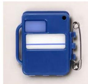
Dosimeter badges - In the first section the window exposes the film to all types of radiation. The second section will block alpha particles and low energy beta particles but let high energy Beta and gamma rays through.
